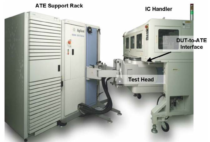
Figure 1: Whole Test System - Tester and Handler Docked Together
